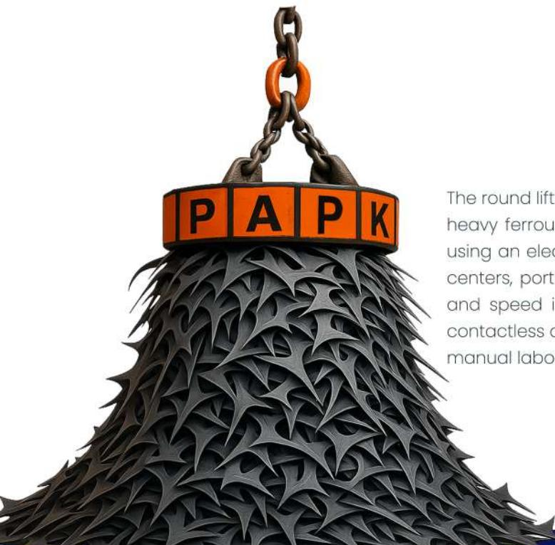
The round lifting magnet is a powerful device designed to lift and move heavy ferrous materials such as steel scrap, billets, and metal sheets using an electromagnetic field. It is widely used in steel mills, recycling centers, ports, and industrial workshops to enhance safety, efficiency, and speed in material handling processes. Key advantages include contactless operation, strong magnetic force, and reduced reliance on manual labor.
