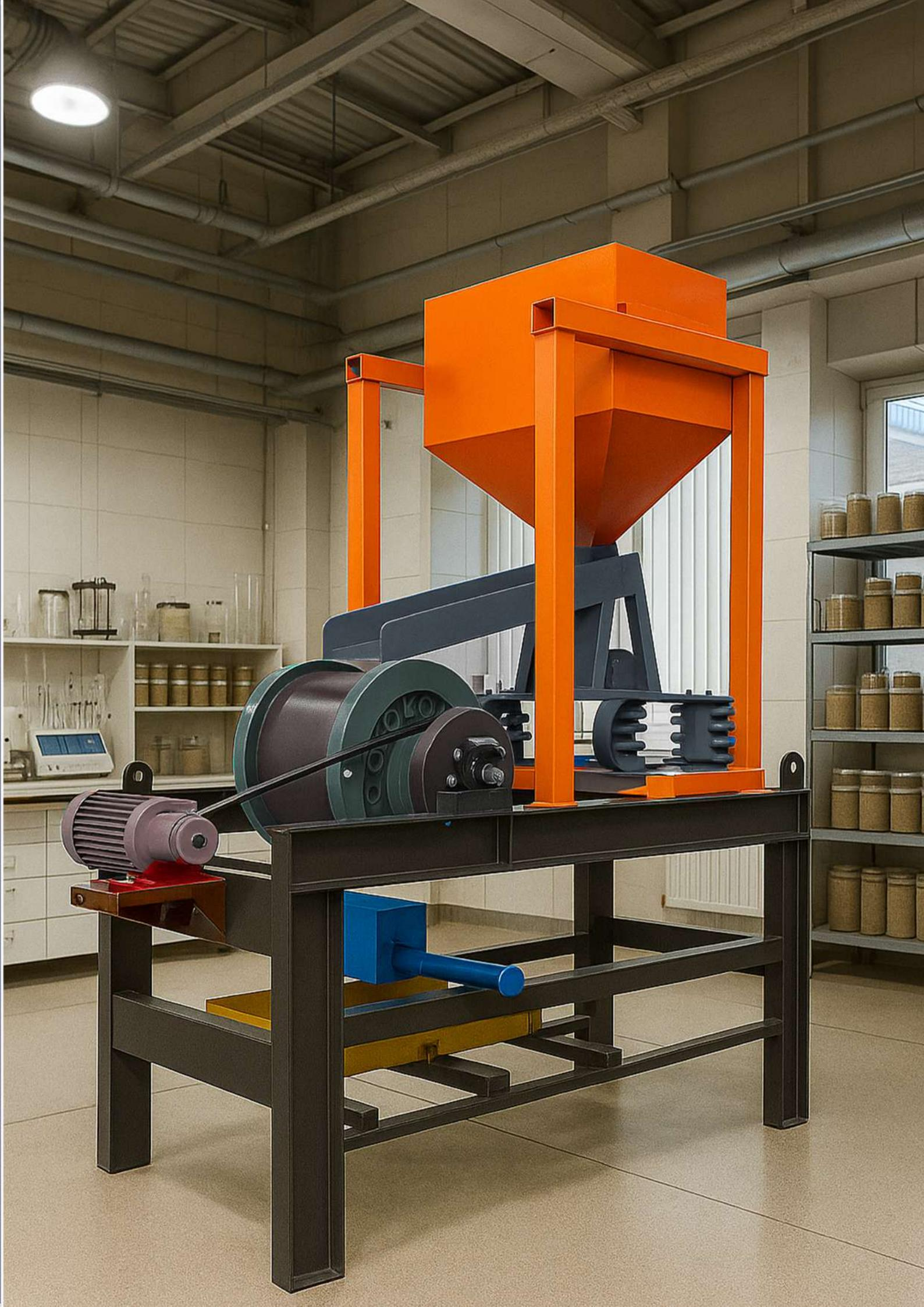
The PAPK Parsian Laboratory Drum Separator is designed for precise magnetic separation of mineral samples in both wet and dry modes.
